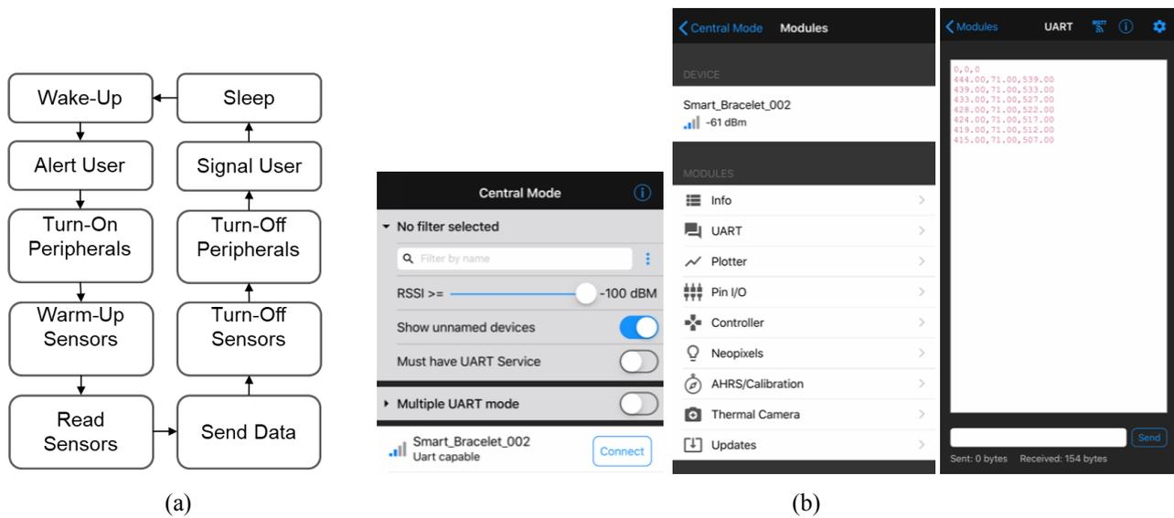
Figure 5: (a) Flow chart for the smart wristband program showing major steps. (b) Screenshots showing the BlueFruit smart app on iPhone XS Max. From left to right: Main page showing smart wristband (Smart\_Bracelet\_002), page after the connection has been established, and receiving data from the smart wristband sensors.
