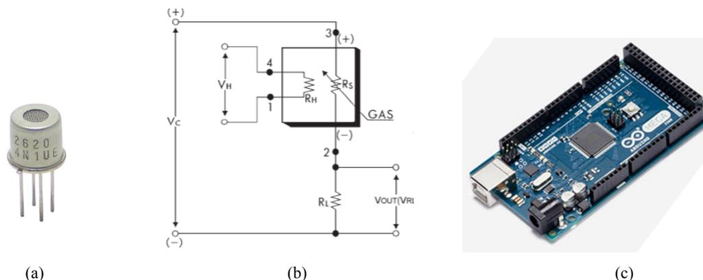
Figure 1: (a) A Figaro 2620 metal oxide semiconductor VOC sensor [23]. (b) A connection to the four pins of the sensors, two pins connecting to an internal heating element and remaining two pins to the sensing element. The sensing element is connected in series with a load resistor ( $R_L$ ) [23]. (c) An Arduino Mega microcontroller.
