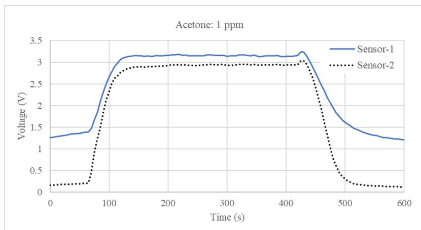
Figure 3: A sample sensor reading showing one complete test cycle with 1 ppm of acetone.
