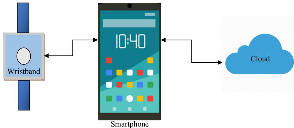
Figure 6: Block diagram showing the overall system architecture that includes the smart wristband, smartphone, and cloud.
