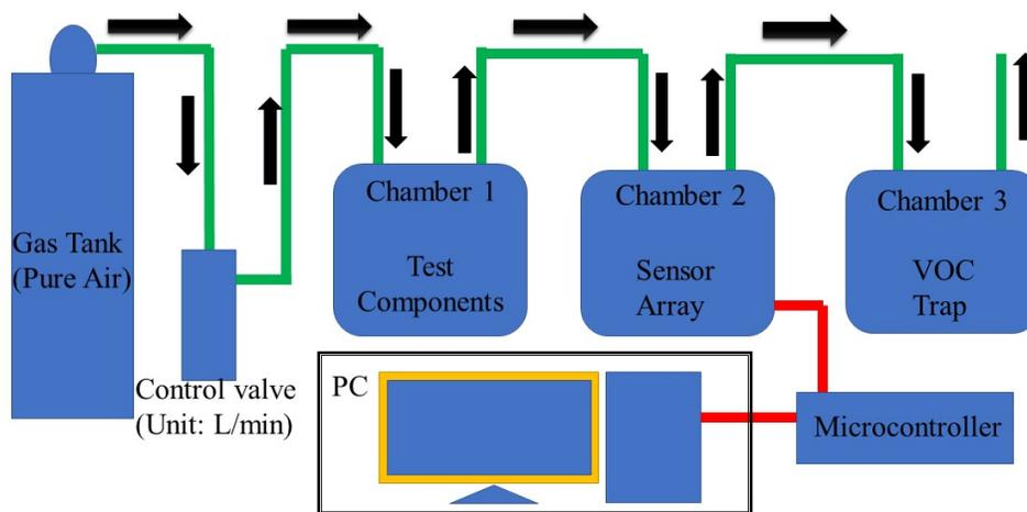
Figure 2: Test setup showing a series connection of air tank, flow control valve, air-tight glass chambers for VOC introduction and sensor array, and a VOC trap. The sensor array connects to a microcontroller which reads the sensors and feeds data to the PC during training. During testing with the trained algorithm implemented in the microcontroller, the PC was used as a serial monitor to observe and save the classification results.
