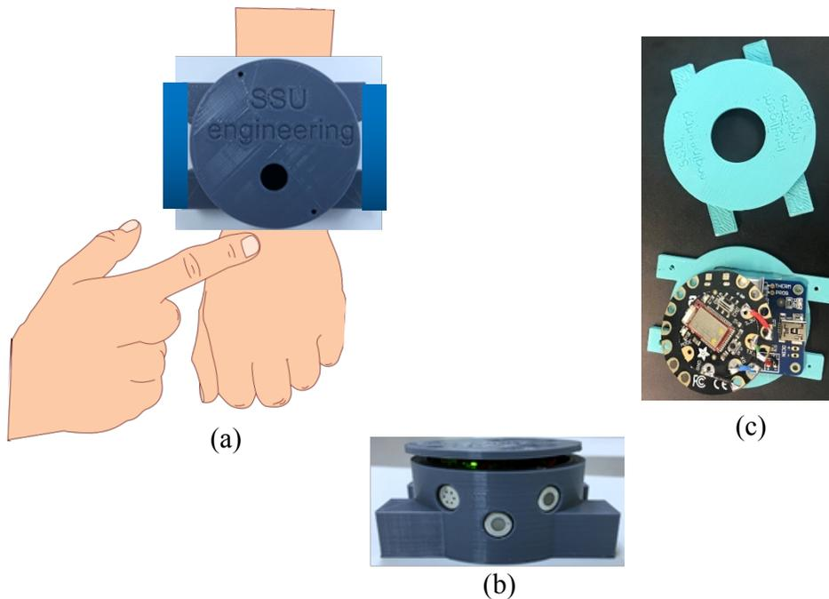
Figure 4: Two versions of wearable smart wristband prototype. (a) Initial version. (b) Side-view of the wristband in (a) showing sensors. (c) Improved version in development.
